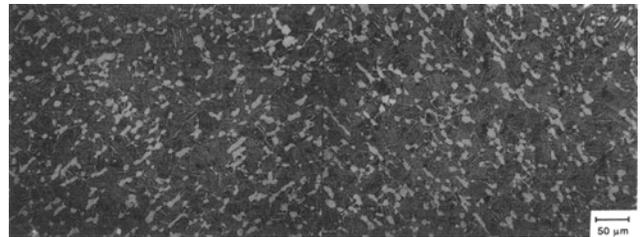
**Fig. 4(b)** Micrograph from face B in a set 2 hammer-forged coupon (annealed at 998 °C).
