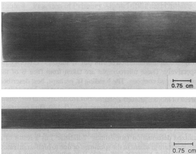
**Fig. 3** Bands observed macroscopically on faces B and C (see Fig. 4) in a set 1 hammer-forged coupon annealed at 968 °C ( $T_{\beta} - 41$  °C).
