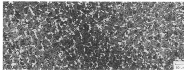
**Fig. 5(b)** Microstructure of face B observed in a set 4 press-forged coupon (annealed at 993 °C).
