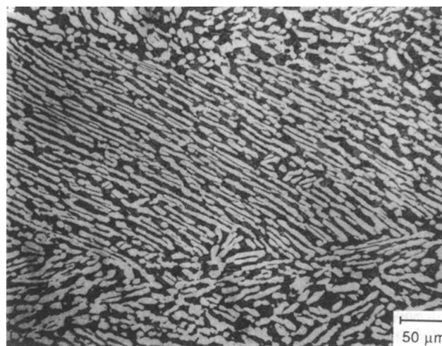
**Fig. 8** Microstructure of the coupon before hammer or press forging but subsequent to heating for 2 hr at 954 °C ( $T_{\beta}-55$  °C).
