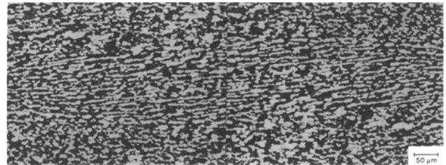
**Fig. 4(a)** Microstructural banding observed in a set 1 hammer-forged coupon (annealed at 968 °C). Banded structures observed here on face B are parallel to the z-direction.
