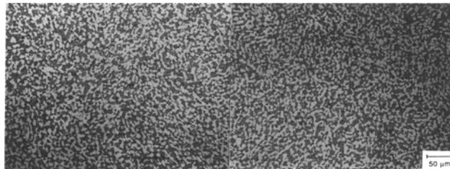
**Fig. 7** Microstructure of face A in a set 1 hammer-forged coupon (annealed at 968 °C).
