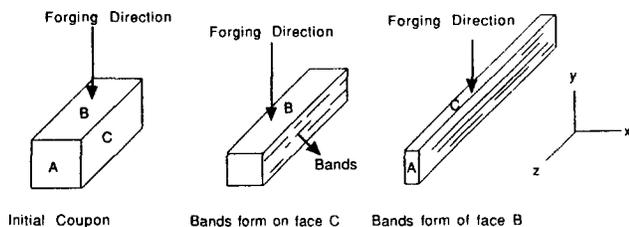
**Fig. 6** Bands observed subsequent to forging on face B and face C in a set 1 hammer-forged coupon (annealed at 968 °C).
