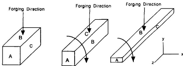
**Fig. 2** Hammer and press forging on faces B and C of coupons.
