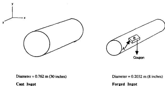
**Fig. 1(a)** Orientation of the coupons that were cut from the ingots.
