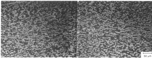
**Fig. 5(a)** Microstructure of face B observed in a set 3 press-forged coupon (annealed at 968 °C).
